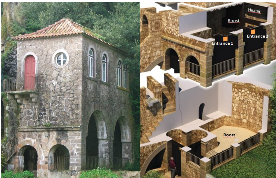
Figure 26. A photograph of the new roost building, along with a cutaway graphic showing the location of the roost, the entrances, and the location of the heaters.
