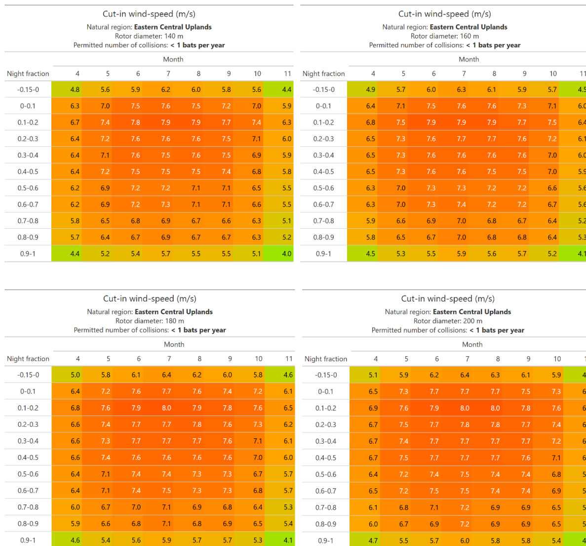
Fig. 21: Cut-in wind speeds (m/s) for an allowable collision mortality of < 1 individual per year for the Eastern Central Uplands at wind turbines with rotor diameters of 140–200 m.
