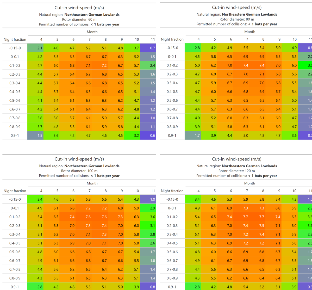
Fig. 16: Cut-in wind speeds (m/s) for an allowable collision mortality of < 1 individual per year for the Northeastern German Lowlands at wind turbines with rotor diameters of 60–120 m.
