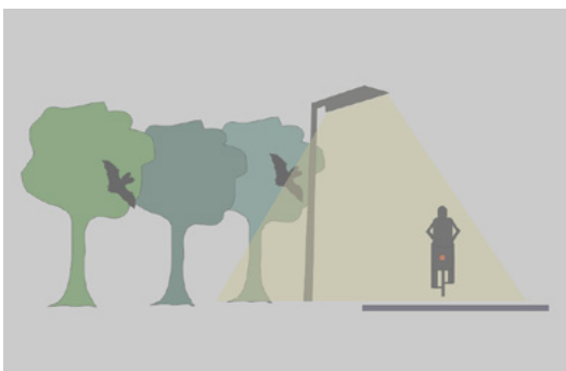
Figure 5.4. Avoidance of light trespass by installing shielded luminaries. Left – conventional luminaire with light spillage into the adjacent forest habitat, right – shielded luminaire that focuses the light cone only on the area where it is needed (© H. LIMPENS).
