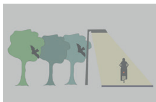
Figure 5.4. Avoidance of light trespass by installing shielded luminaires. Left – conventional luminaire with light spillage into the adjacent forest habitat, right – shielded luminaire that focuses the light cone only on the area where it is needed (© H. LIMPENS).
