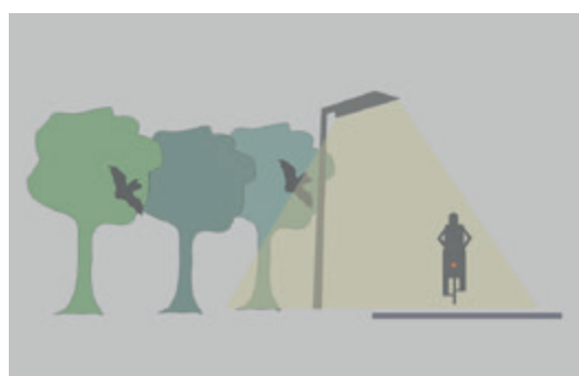
Figure 5.4. Avoidance of light trespass by installing shielded luminaires. Left – conventional luminaire with light spillage into the adjacent forest habitat, right – shielded luminaire that focuses the light cone only on the area where it is needed (© H. LIMPENS).
