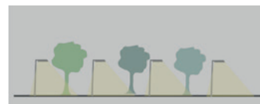
Figure 5.5. Combined effect of shielded luminaires and short poles on reducing light trespass. First picture – unshielded luminaires, second – luminaires with shields. The third picture shows shielded luminaires on short poles which cut-off light trespass and keep adjacent areas dark (© H. LIMPENS).
