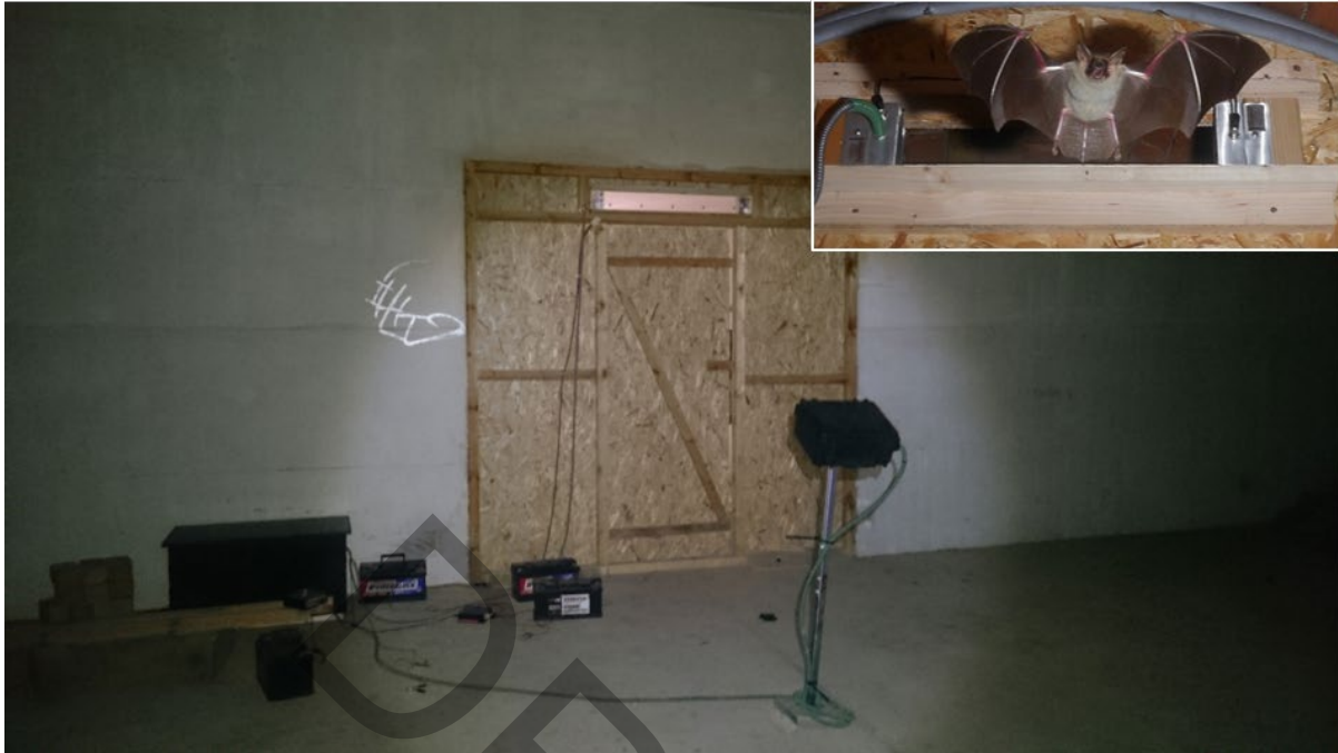
Fig. 2: Lightbarrier system with photo trap (ChiroTEC, Lohra, Germany) maintained with car batteries in a former military bunker in the Nossentiner/Schwinzer Heide (Germany). Upper right photo: greater mouse-eared bat ( Myotis myotis ) entering the photo trap © M. Fritze, AG Kerth).
